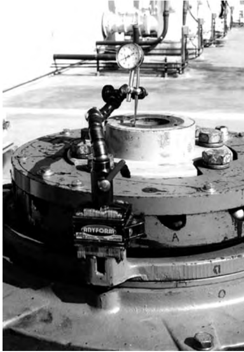
FIGURE 21.35 Measuring runout on the upper hub.
