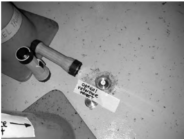
FIGURE 16.57 Permanent floor target.
