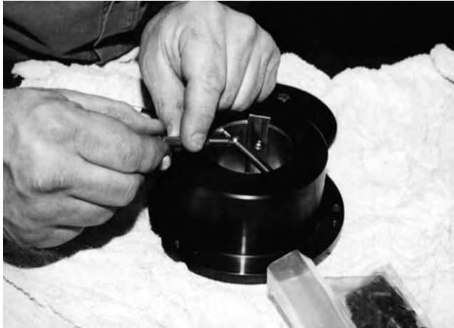
FIGURE 4.24 Measuring bore of coupling hub with a snap gauge.
