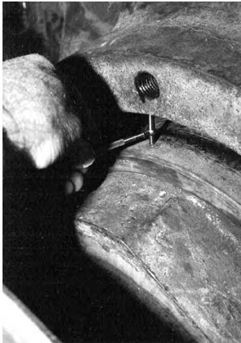
FIGURE 5.16 Snap gauge used to measure stuffing box clearance.
