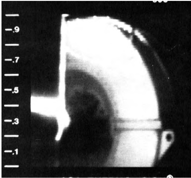
FIGURE 16.7 Thermal image of compressor end casing.
