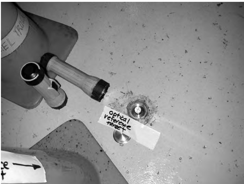
FIGURE 20.15 A permanent floor monument.
