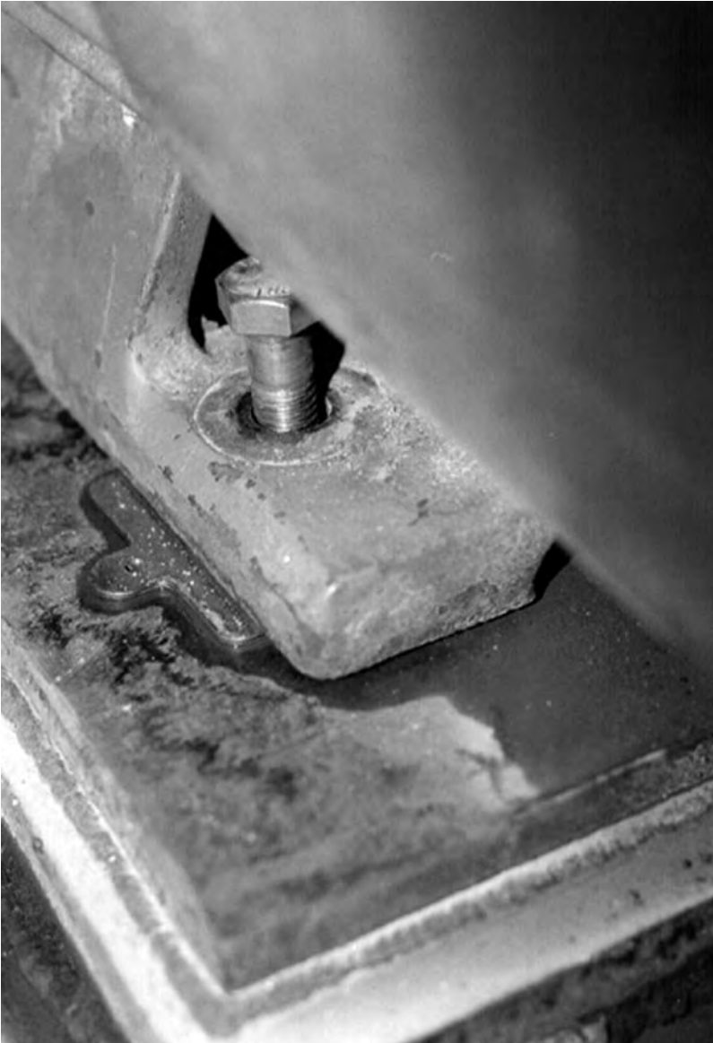
FIGURE 7.4 Observing bolt clearances at a machine foot.
