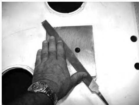
FIGURE 3.35 Removing burrs with a flat file.
