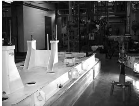
FIGURE 3.43 Jig transit observing scale targets.
