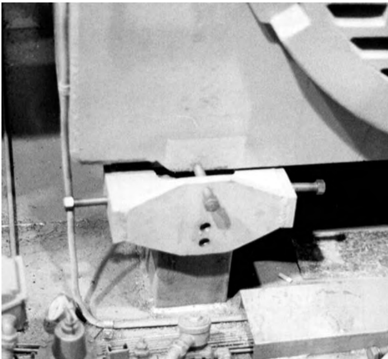
FIGURE 7.24 Bolt-on pusher/puller device bolted to frame rail and ready to push or pull in the sideways direction or push in the axial direction.
