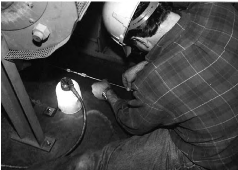
FIGURE 16.12 Measuring between two tooling balls with inside micrometer.
