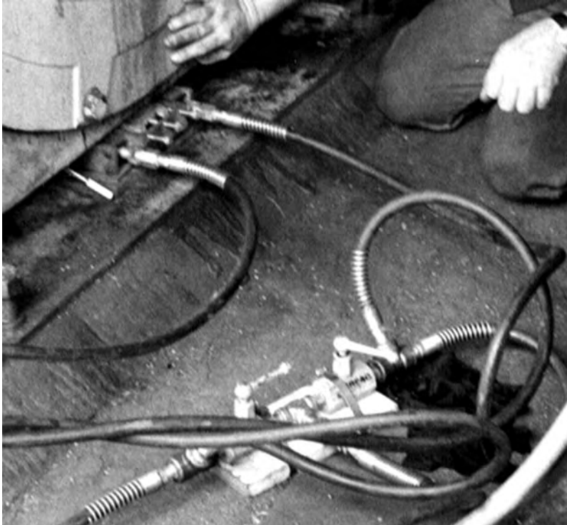
FIGURE 7.17 Hydraulic machinery lifting and lateral positioning device. (Courtesy of Murray & Garig Tool Works, Baytown, TX. With permission.)
