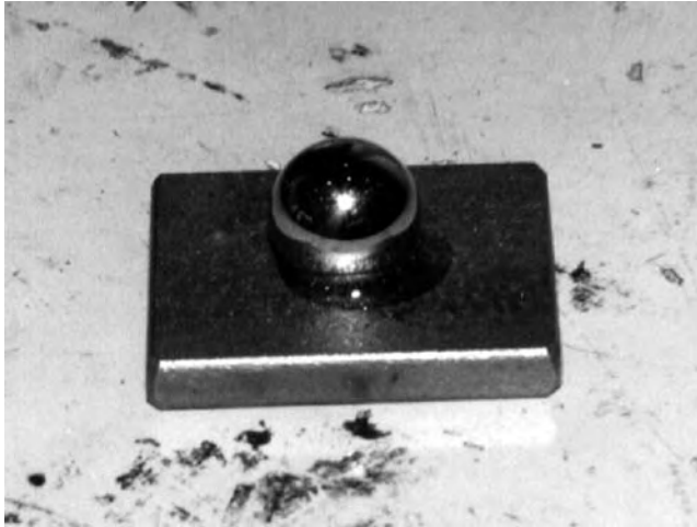
FIGURE 16.9 Tooling ball fabricated from 0.5 in. steel ball and 1.5 in. \times 1.5 in. \times 0.25 in. steel plate with the ball welded to the plate.
