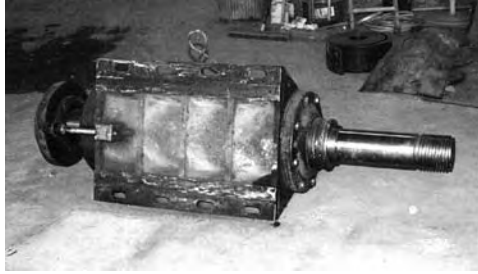
FIGURE 5.35 Underside of pump bearing housing frame that needed resurfacing die to improper contact with its frame.
