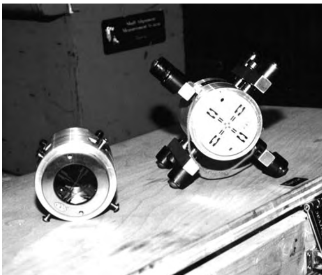
FIGURE 19.11 Bore sighting target fixtures.
