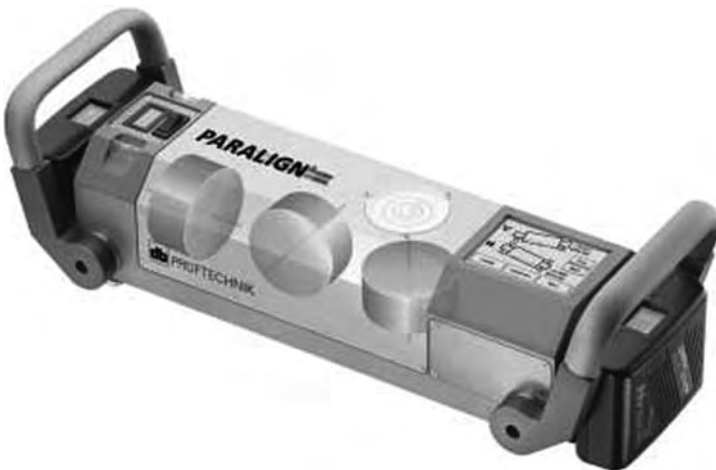
FIGURE 20.31 Paralign internals showing the three ring laser gyroscope in orthogonal positions. (Courtesy of Prüftechnik, Ismaning, Germany. With permission.)
