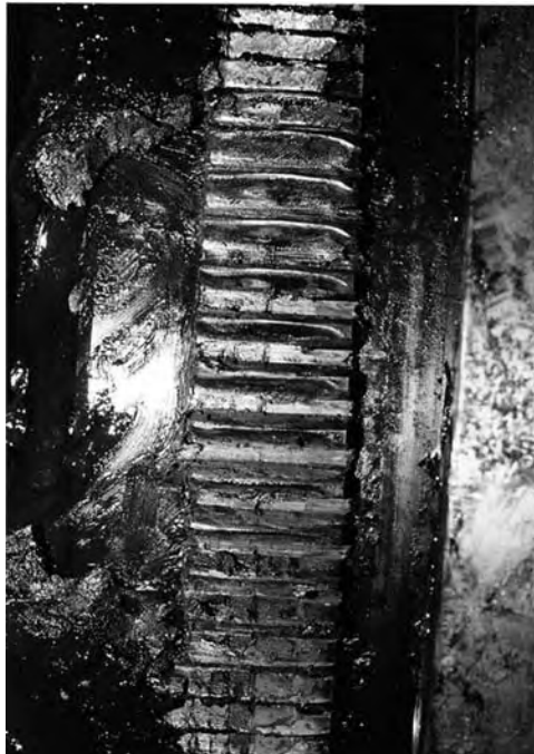
FIGURE 5.20 Excessively worn gear coupling.
