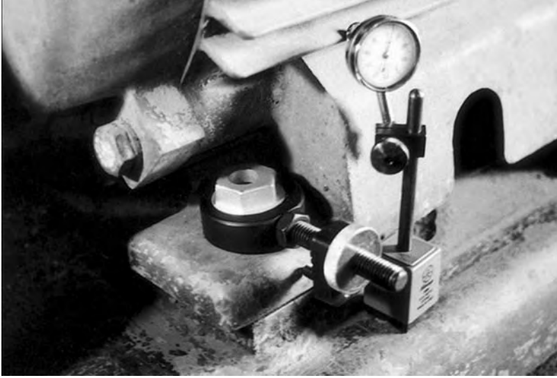
FIGURE 7.25 Portable jack bolt attached to machine case. (Courtesy of Posi Lock Puller, Inc., Cooperstown, ND. With permission.)
