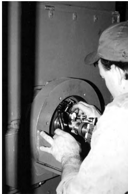
FIGURE 5.29 Measuring runout on a stub shaft.
