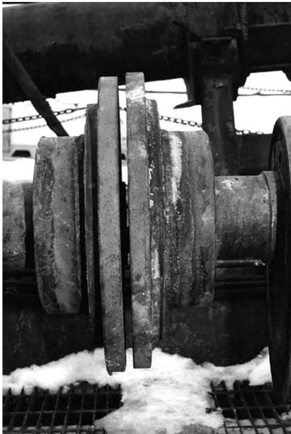
FIGURE 6.3 Misalignment visible by eye.
