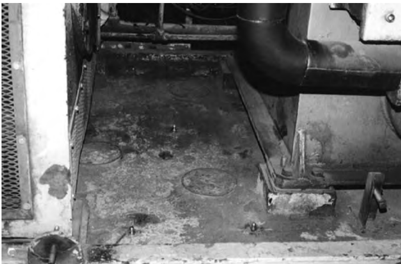
FIGURE 16.18 Tooling ball setup to measure inboard bearings on motor and hydraulic clutch.
