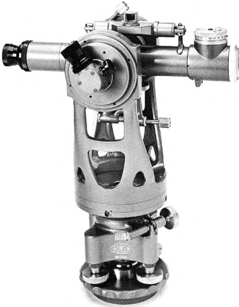
FIGURE 20.5 Telescopic transit square. (Courtesy of Brunson Instruments Co., Kansas City, MO. With permission.)
