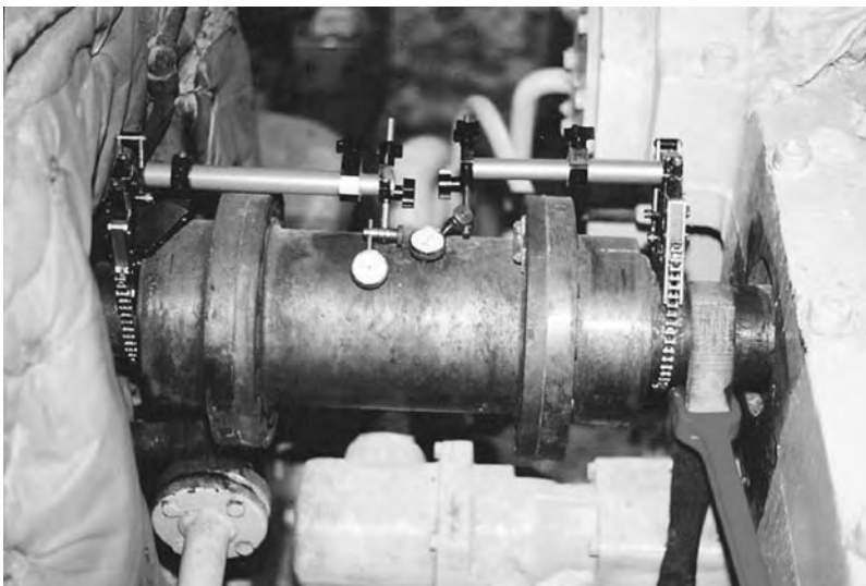
FIGURE 13.4 Shaft to coupling spool method employed on gear coupling with measurements taken on the spacer (spool).
