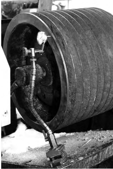
FIGURE 5.32 Measuring face runout on a multi-V sheave.
