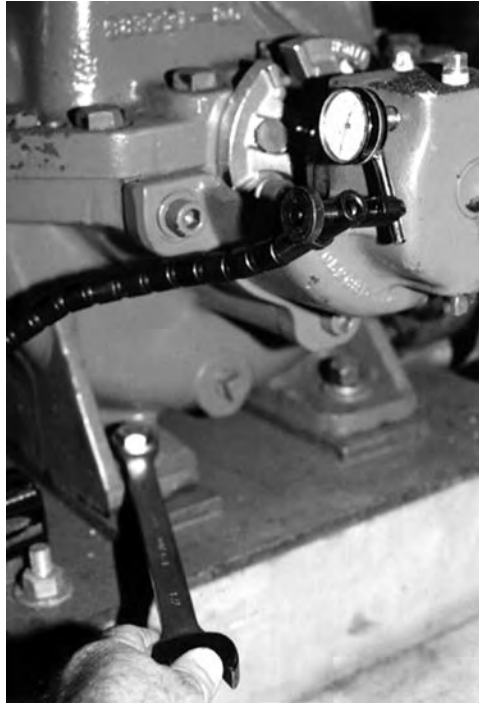
FIGURE 3.74 Alternate piping stress check using magnetic base and indicator to observe case movement when foot bolts are loosened with piping attached.
