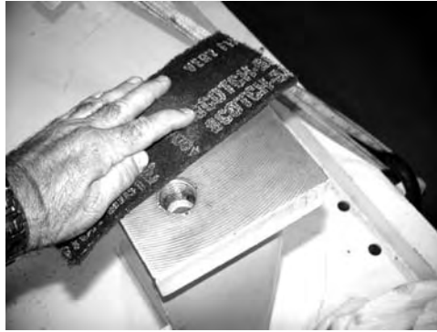
FIGURE 3.34 Cleaning the top surfaces of each mounting point.
