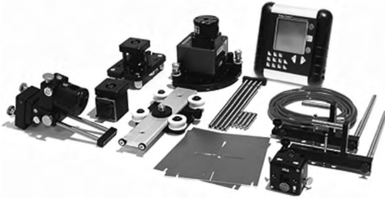
FIGURE 20.20 Damalini Model D670 roll parallelism measurement system. (Courtesy of Damalini, Molndal, Sweden. With permission.)
