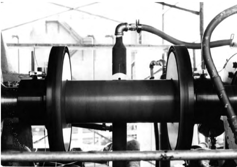
FIGURE 16.34 Water-cooled stands with proximity probes observing position of coupling hubs. (Courtesy of Charlie Jackson, Texas City, TX. With permission.)
