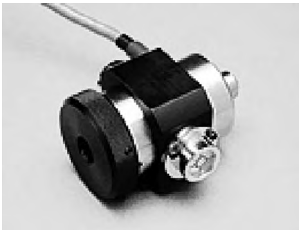
FIGURE 20.28 Hamar Model T-212 4 axis target. (Courtesy of Hamar Laser Instrument Co., Danbury, CT. With permission.)
