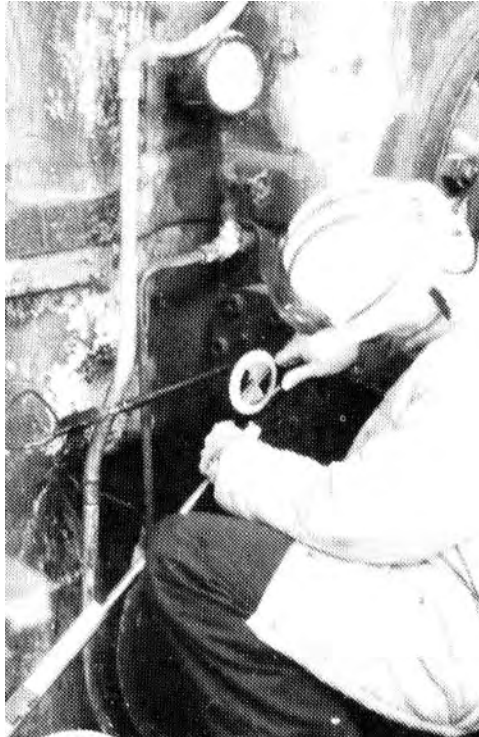
FIGURE 16.14 Measuring the angle with the Acculign inclinometer.
