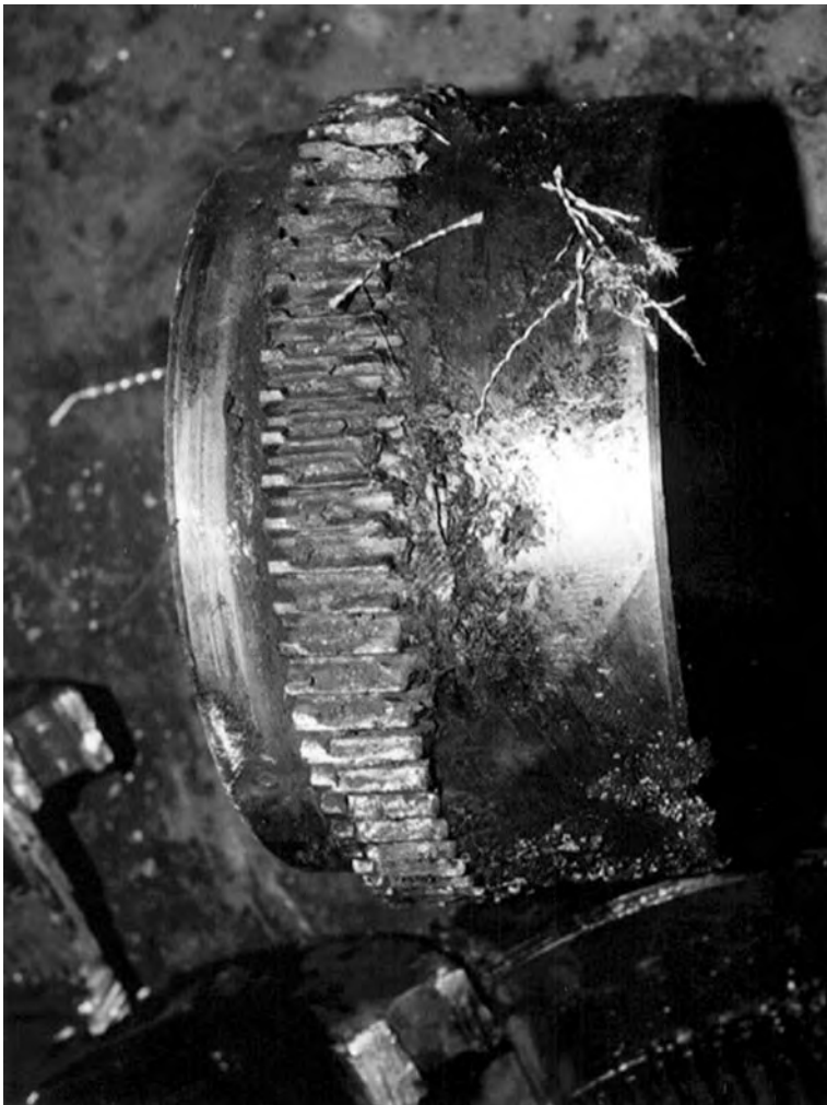
FIGURE 1.8 Worn gear coupling hub.
