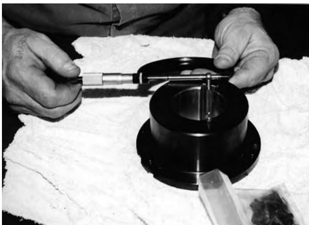
FIGURE 4.25 Using an outside micrometer to measure the snap gauge.
