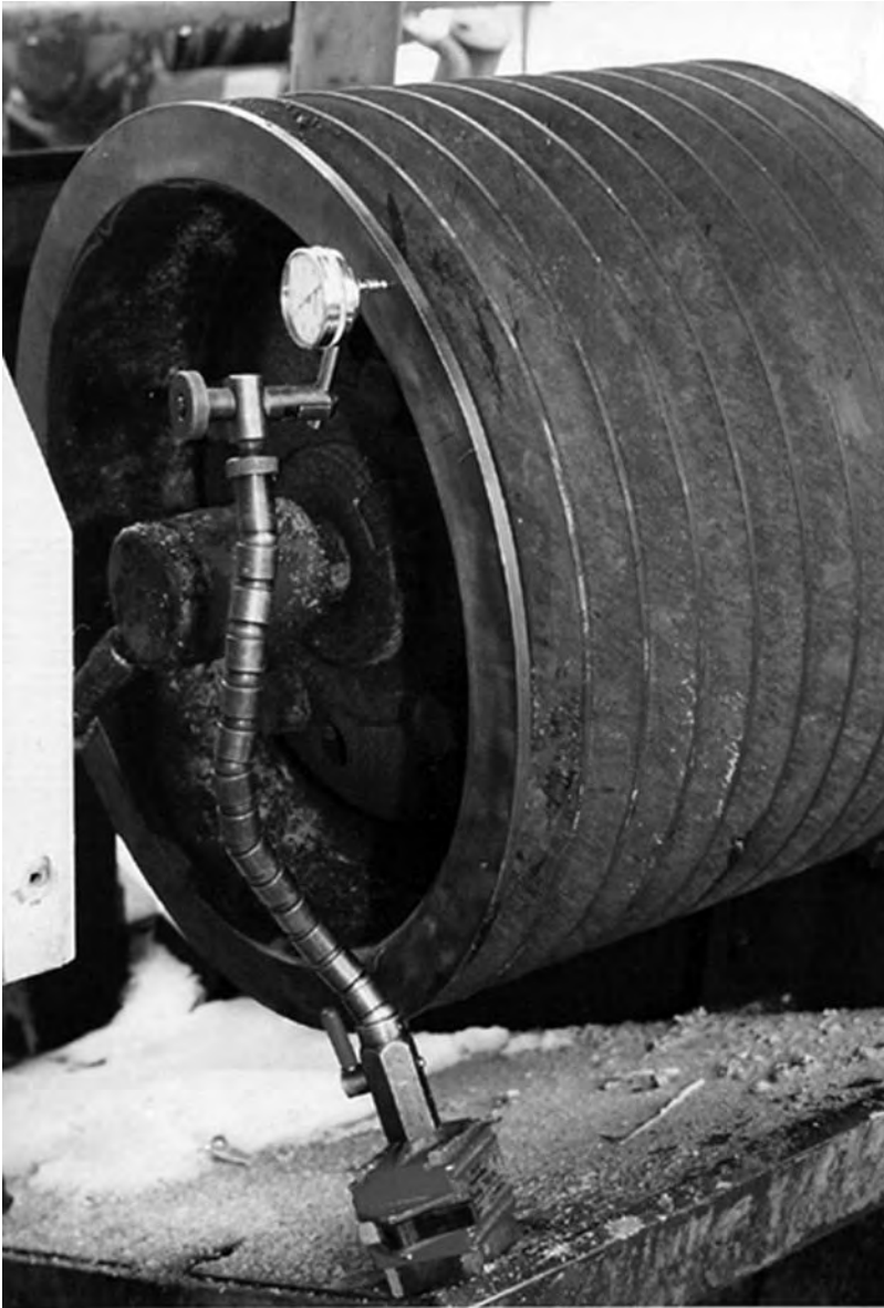
FIGURE 18.13 Face runout check on sheave.
