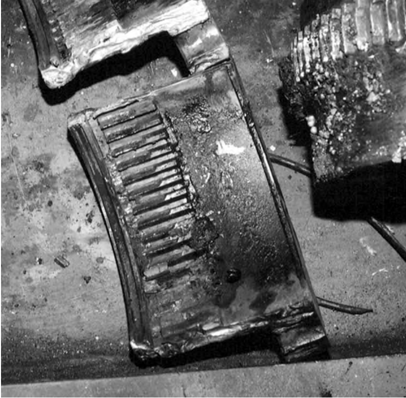
FIGURE 1.5 Excessively worn gear coupling due to operation under moderate misalignment conditions.
