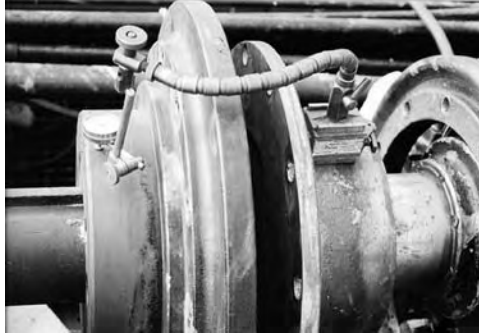
FIGURE 5.26 Measuring runout on rubber time coupling hub.
